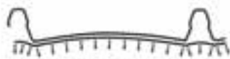
The rigid shape of an inflated airbag does not apply pressure to the ribs of secret-fixed cladding or adjacent to supports
