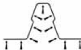
BLUESCOPE LYSAGHT's direct pressure rig uses no air bags and applies pressure uniformly over the entire profile – including the ribs.
